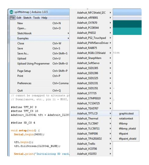
You may need to press the Reset button to reset the Arduino and TFT. You should see a collection of graphical tests draw out on the TFT.
