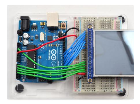
You can connect the seventh pin RST (Reset) to the Arduino Reset line if you'd like. This will reset the panel when the Arduino is Reset. You can also use a digital pin for the LCD reset if you want to manually reset. There's auto-reset circuitry on the board so you probably don't need to use this pin at all and leave it disconnected
