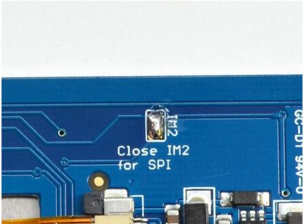
If you really don't want to solder, you can also wire the breakout pin to the 3vo pin, just make sure you don't tie it to 5V by accident! For that reason, we suggest going with the solder-jumper route.
