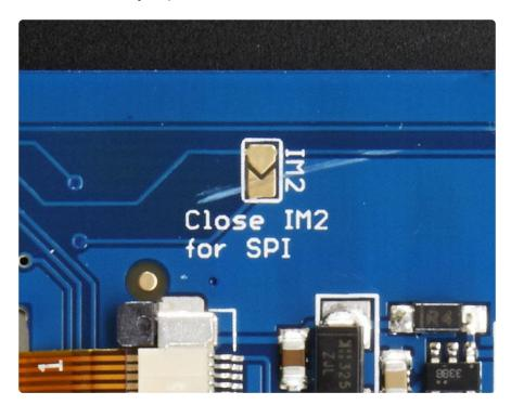
With your soldering iron, melt solder to close the jumper indicated IM2
