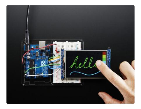
The LCD has a 3.5" 4-wire resistive touch screen glued onto it. You can use this for detecting finger-presses, stylus', etc. You'll need 4 pins to talk to the touch panel, and at least 2 must be analog inputs. The touch screen is a completely separate part from the TFT, so be aware if you rotate the display or have the TFT off or reset, the touch screen doesn't "know" about it - its just a couple resistors!
