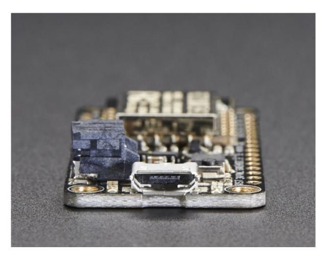
To make it easy to use for portable projects, we added a connector for any of our 3.7V Lithium polymer batteries and built in battery charging. You don't need a battery, it will run just fine straight from the micro USB connector. But, if you do have a battery, you can take it on the go, then plug in the USB to recharge. The Feather will automatically switch over to USB power when its available.
