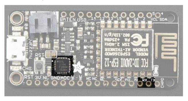
The **TX** pin is the output *from* the module and is 3.3V logic.
