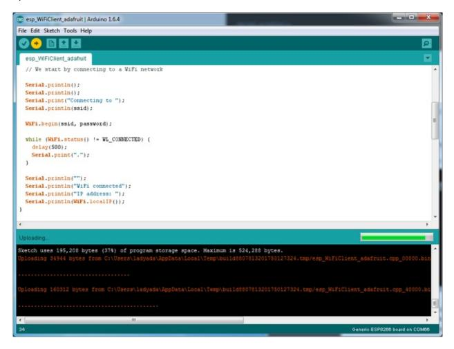
Open up the IDE serial console at 115200 baud to see the connection and webpage printout!
