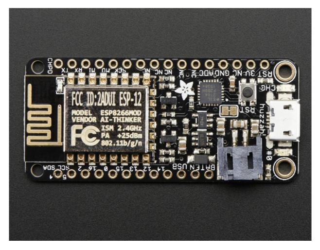
While the Feather HUZZAH ESP8266 comes pre-programmed with NodeMCU's Lua interpretter, you don't have to use it! Instead, you can use the Arduino IDE which may be more familar. **This will write directly to the firmware, erasing the NodeMCU firmware**, so if you want to go back to Lua, use the flasher to re-install it (http://adafru.it/f1O)
