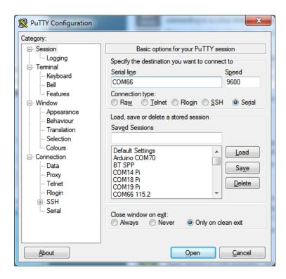
Once the terminal software is connected, click the **Reset** button on the Feather HUZZAH ESP8266 board to reset it and have it print out the welcome message:
