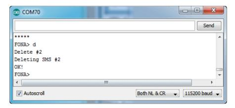
Note that before I deleted SMS #2, so if I read them again, that SMS # will be an empty slot. SMS number #3 doesn't "move slots"!
