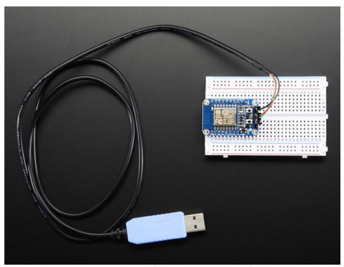
Each module comes pre-loaded with NodeMCU's Lua interpreter (NodeMCU 0.9.5 build 20150318 / Lua 5.1.4 to be specific) (http://adafru.it/inA), you can run commands, and 'save' Lua programs directly to the module's Flash using a USB-Serial converter cable.
