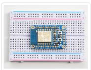
Place the breakout board over the pins so that the short pins poke through the breakout pads
