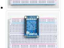
Place the breakout on the breadboard facing down
