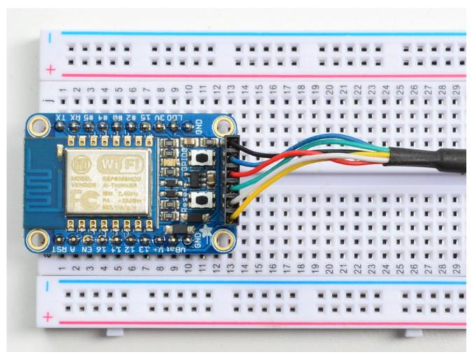
If using a console cable, connect the black wire to ground, red wire to V+, white wire to TX and green wire to RX
