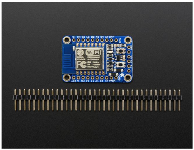
Each order comes with one assembled and tested HUZZAH ESP8266 breakout board, and a stick of 0.1" header that you can solder on and plug the breakout into a breadboard. A soldering iron and solder is required for that, and aren't included. **You'll also need a USB-serial cable** such as a USB console cable (Windows only) (http://adafru.it/dDd), FTDI Friend (any OS) (http://adafru.it/284), or FTDI cable (any OS) (http://adafru.it/70)to upload software to the HUZZAH ESP8266!
