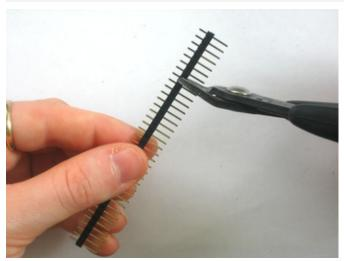
Next its time to make the headers for the jumper, servos and arduino.
