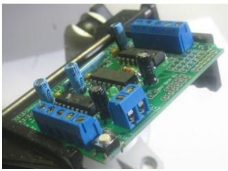
The 2 3-pin pieces go in the servo connections in the top left corner. The 2-pin piece goes in the PWR jumper in the bottom center.
