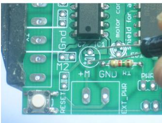
Place the two 47uF remaining electrolytic capacitors, C7 and C8
