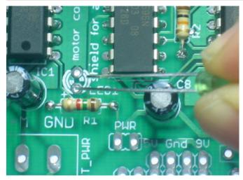
Next is the 3mm LED used to indicate motor power. LEDs are polarized, just like capacitors, and the long lead is the positive (+) lead.
