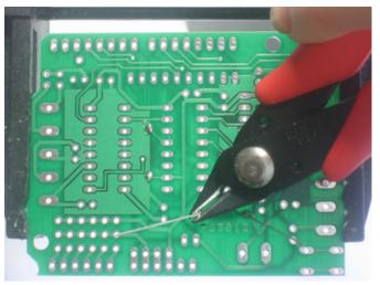
Clip the long leads, just above the solder joint using diagonal cutters.
