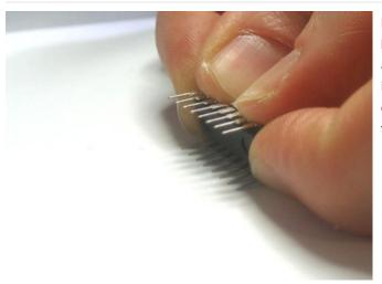
Next are the three integrated circuits (ICs) IC1, IC2 and IC3. When ICs come from the factory, the legs are angled out somewhat which makes it difficult to insert them into the PCB. Prepare them for soldering by gently bending the legs against a flat tabletop so that they are perfectly straight.
