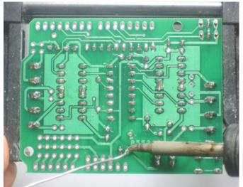
Solder in the 3 pieces of header and the three terminal blocks.
