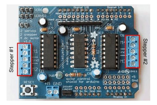
AF\_Stepper Stepper1(48, 1); // A 48-step-per-revolution motor on channels 1 & 2 AF\_Stepper Stepper2(200, 2); // A 200-step-per-revolution motor on channels 3 & 4
