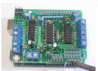
Solder in each pin of the header.
