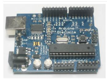
Next, place the 8-pin and 6-pin headers into the Arduino board. This will make sure that the headers are perfectly lined up. Make sure the Arduino is not plugged in or powered!
