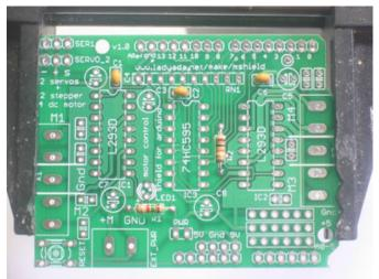
Next place the three yellow ceramic capacitors **C4**, **C2** and **C6**. Ceramic capacitors are not polarized so you can put them in "either way" and they work fine.
