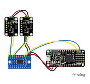
Board 3V to mux VIN (red wire) Board GND to mux GND (black wire) Board SCL to mux SCL (yellow wire) Board SDA to mux SDA (blue wire)
