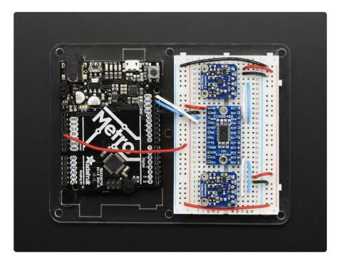
Like all Adafruit breakouts, we put this nice chip on a breakout for you so you can use it on a breadboard with capacitors, and pullups and pulldowns to make usage a snap. Some header is required and once soldered in you can plug it into a solderlessbreadboard. The chip itself is 1.8V - 5V compliant so you can use it with any logic level.
