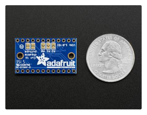
Using it is fairly straight-forward: the multiplexer itself is on I2C address 0x70 (but can be adjusted from 0x70 to 0x77) and you simply write a single byte with the desired multiplexed output number to that port, and bam - any future I2C packets will get sent to that port. In theory, you could have 8 of these multiplexers on each of 0x70-0x77 addresses in order to control 64 of the same-I2C-addressed-part.
