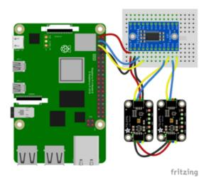
Pi 3V to mux VIN (red wire) Pi GND to mux GND (black wire) Pi SCL to mux SCL (yellow wire) Pi SDA to mux SDA (blue wire) TSL25911 SDA to mux SD0 TSL25911 SCL to mux SC0 TSL25911 VIN to mux VIN TSL25911 GND to mux GND
