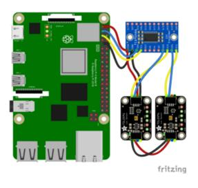
Pi 3V to mux VIN (red wire) Pi GND to mux GND (black wire) Pi SCL to mux SCL (yellow wire) Pi SDA to mux SDA (blue wire) TSL25911 SDA to mux SD0 TSL25911 SCL to mux SC0 TSL25911 VIN to mux VIN TSL25911 GND to mux GND
