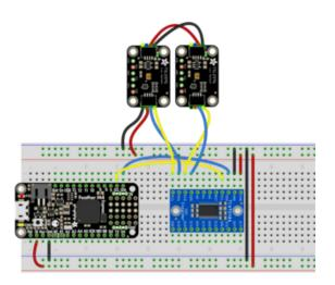
Board 3V to mux VIN (red wire) Board GND to mux GND (black wire) Board SCL to mux SCL (yellow wire) Board SDA to mux SDA (blue wire)
