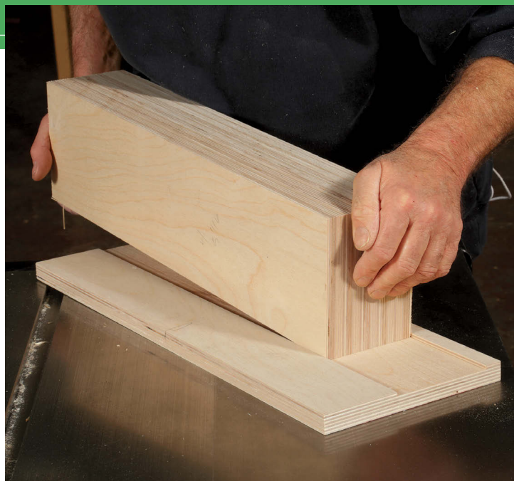
Dado the uprights to locate the bridge. The bridge should fit snugly. Position the dado so the bridge rides above the rip fence. You want the jig to ride on the saw table, not the fence. After this, drill the holes for hex bolts.
