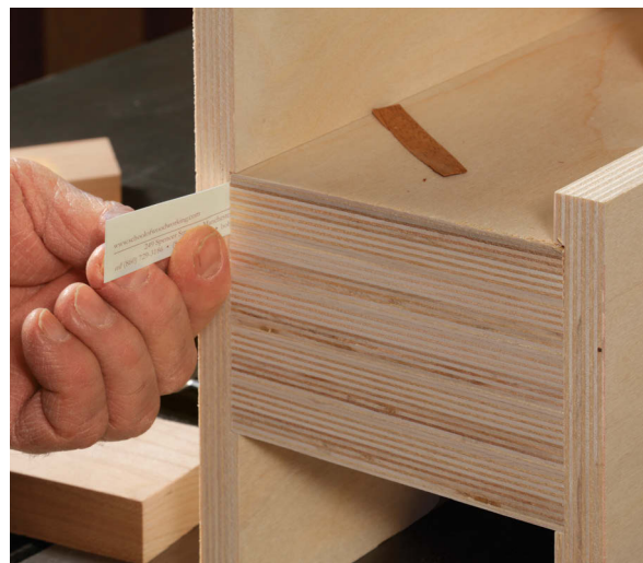
Dry-fit the jig to see if the tall upright needs shimming. It is critical that the tall upright is perfectly square to the table, since any inaccuracy here will impact your tenons. Shim if necessary (right). The short upright just gets screwed in place after getting predrilled for the pressure bar's hex bolts.
