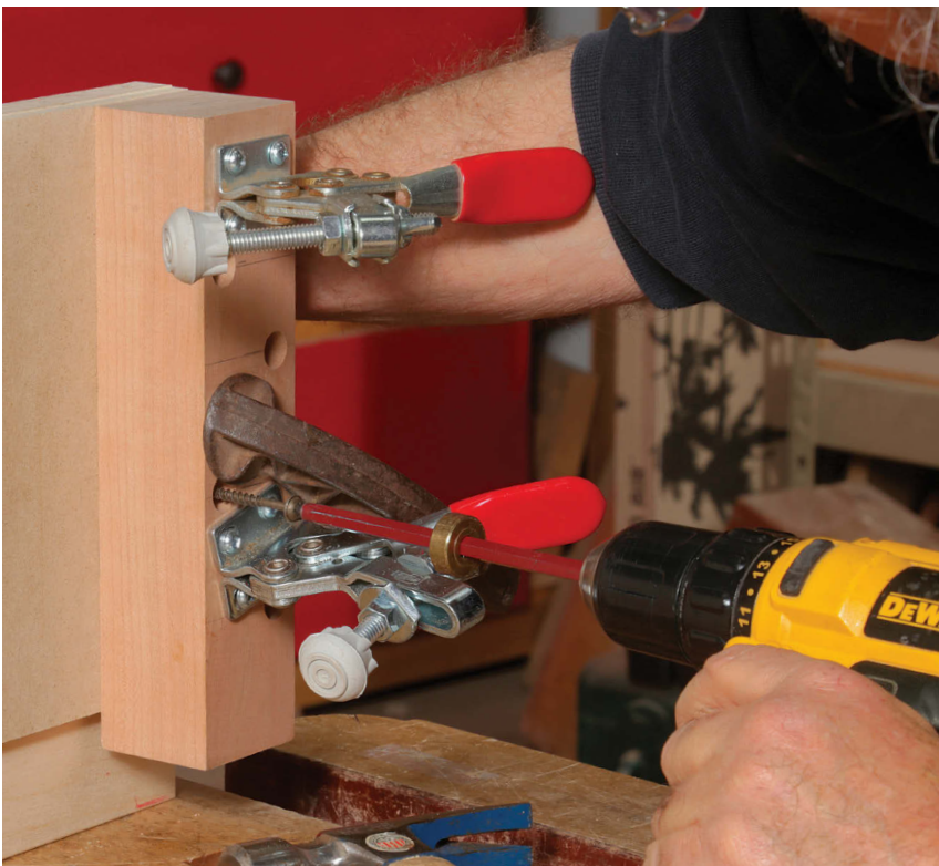
Install the vertical support and toggle clamps. This block both supports the workpiece and holds toggle clamps. Install it square, and mount it about 1 in. above the saw table (above). Then double-stick tape the zero-clearance sacrificial strip in place (right). This strip backs up the workpiece, limiting tearout on the back of the cut.
