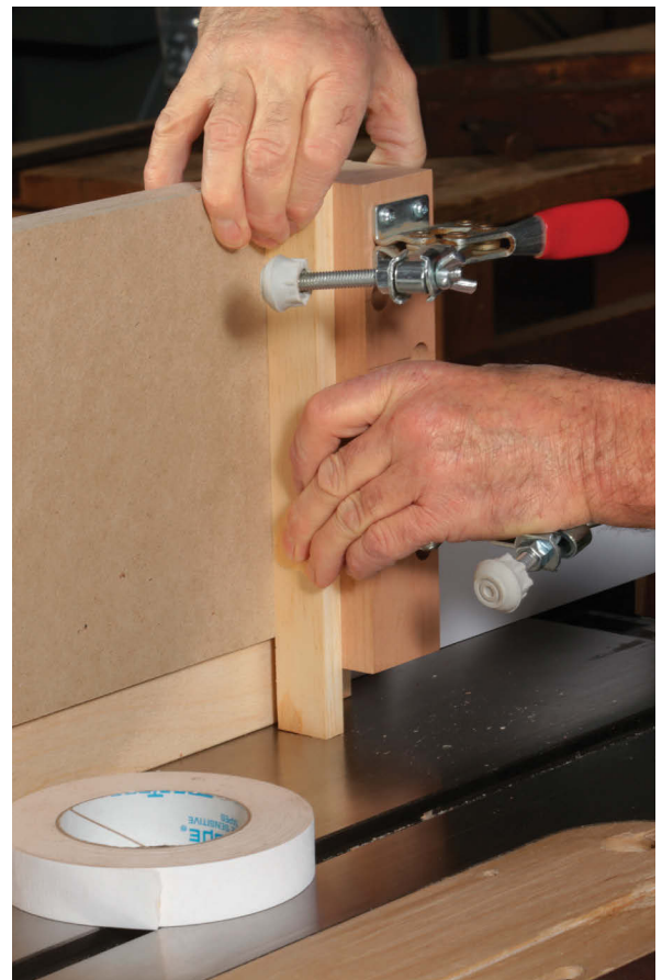
Install the vertical support and toggle clamps. This block both supports the workpiece and holds toggle clamps. Install it square, and mount it about 1 in. above the saw table (above). Then double-stick tape the zero-clearance sacrificial strip in place (right). This strip backs up the workpiece, limiting tearout on the back of the cut.
