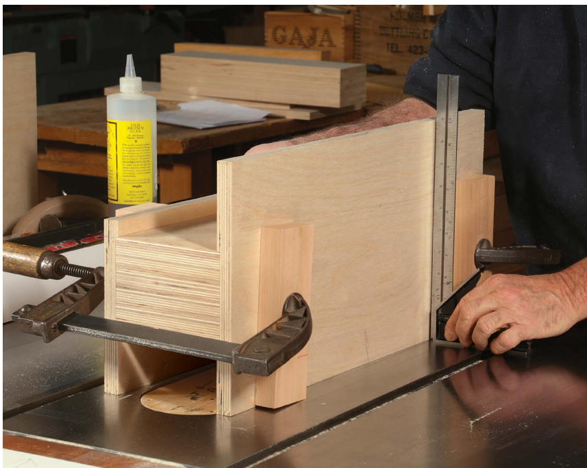
Dry-fit the jig to see if the tall upright needs shimming. It is critical that the tall upright is perfectly square to the table, since any inaccuracy here will impact your tenons. Shim if necessary (right). The short upright just gets screwed in place after getting predrilled for the pressure bar's hex bolts.
