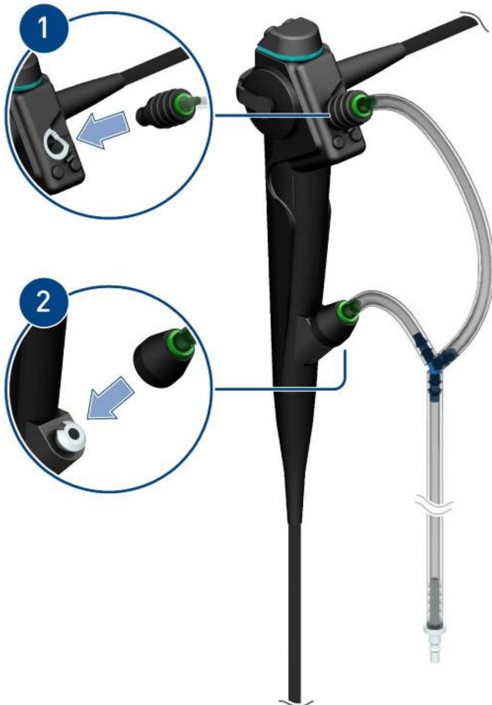
Figure 3.24 Connecting BF-30 Scopes
