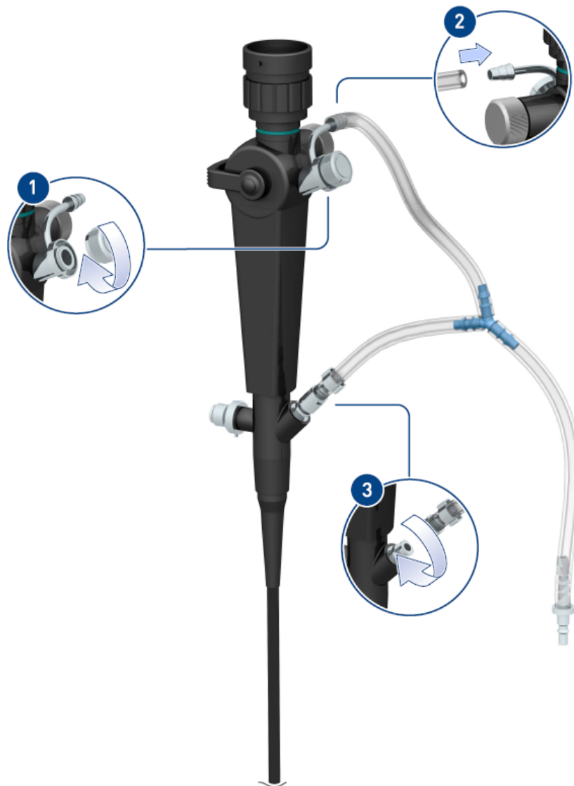
Figure 3.39 Connecting Pentax FB scopes
