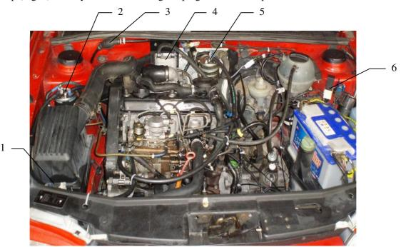
Fig. 2. **Displacement of one-tank system components in engine compartment**: 1 – valve; 2 – original fuel filter; 3 – fuel hand pump; 4 – heat exchanger; 5 – fuel heater/filter; 6 – relays
