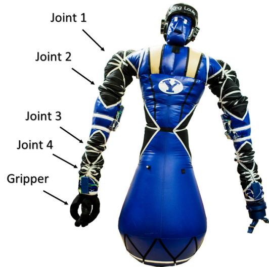
Fig. 1: King Louie is a fully inflatable, pneumatically actuated platform with four degrees of freedom in each arm.
