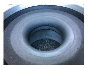
Figure 11: Coated compressor housing after 150,000 miles in service
