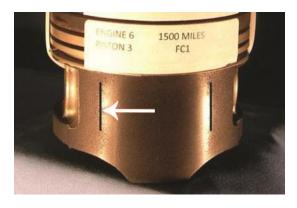
Figure 3B: Stribeck Fitting Results, Armor AAPC; reduced IPWC, larger contact area, extended oil leak path, reduced peak stress on oil film, limited rocking room, nearly scratch free while running alongside Figure 3A piston
