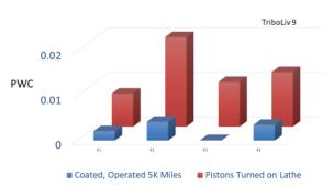
**Figure 8:** Piston to Wall Clearance (PWC) was corrected by AAPC after turning piston skirts to undersize straight on a lathe, coating them to fit. Coated pistons operated 5000 miles before remeasuring.
