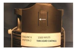
Figure 3A: Thin coating with normal IPWC. Narrow contact area, foreign particle scratches visible
