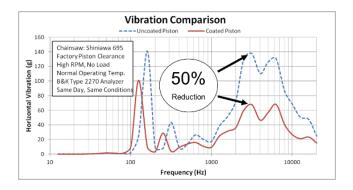
Figure 4A: Slick+ AAPC reduces Vibration
