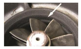
**Figure 9:** Rotor bedded into soft coating - perfect seal (zero clearance and zero friction) after 150,000 miles
