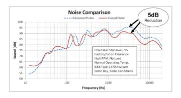
Figure 4B: SlickCC AAPC reduces Noise ~ 5db across audible spectrum
