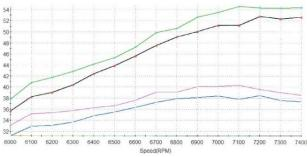
Figure 6: A-B dyno runs, same day. SlickCC AAPC coated 2 stroke pistons made approximately 7% more power across the rpm range
