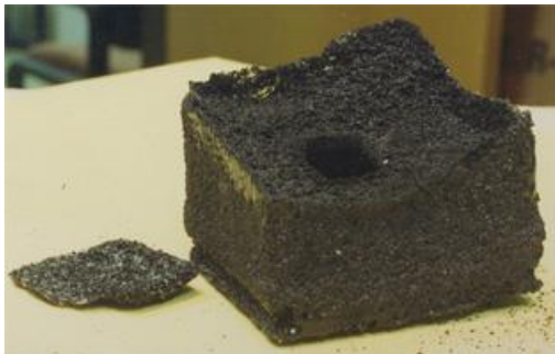
One of the first attempts at making an object with selective laser sintering.
