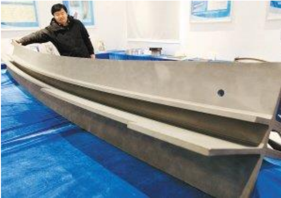
3D printed, titanium central wing spar
