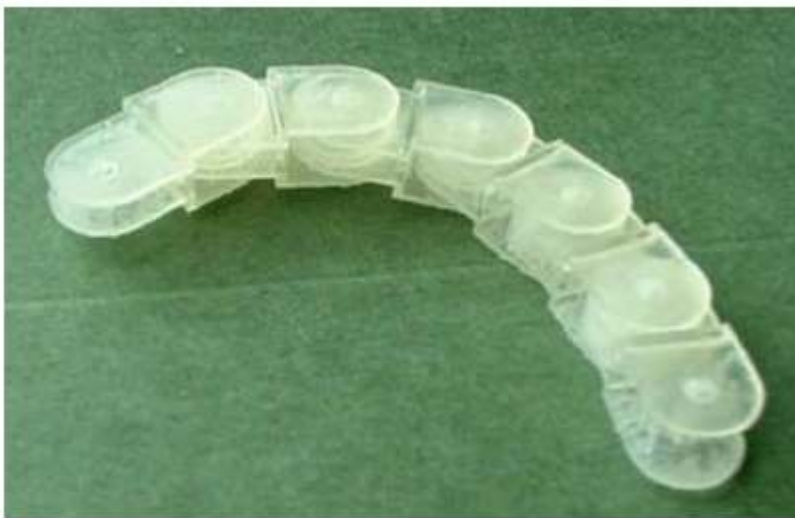
Pulley-driven snake-like robot Source: Gibson.
