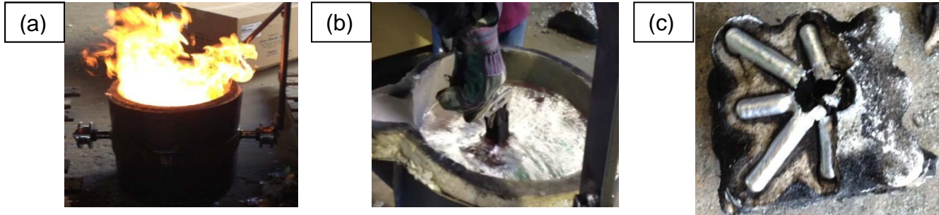
Figure 22: Trial 2 (a) Pre-Heat Mold, (b) Mold Dipped in Molten Metal Pool (c) Opened Shell
