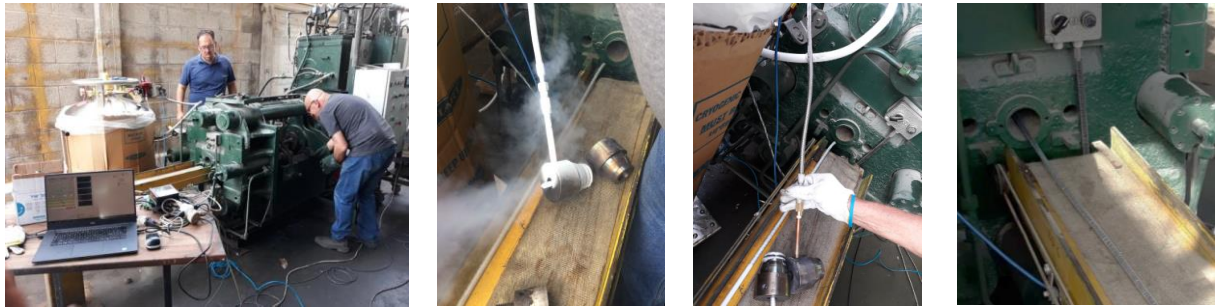
Figure 7. Experimental trials at Alubin: (a) nitrogen tank and extrusion press, (b) 3 mm design after trials, (c) 1.5 mm design after trials, (d) profile at the die exit
