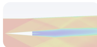
DLR SCRAMJET, Mach 2. Turbulent, H 2
