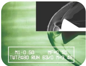
Re-entry capsule with counter-flow jet, Mach 3.5, Turbulent, Air as ideal-gas (Daso case)
