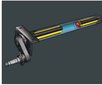
Rubber torsion "independent suspension" axles
