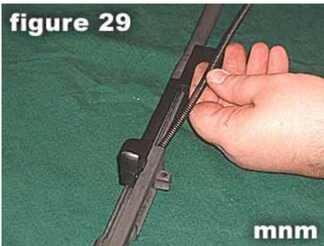
29) Feed recoil spring guide into receiver.
