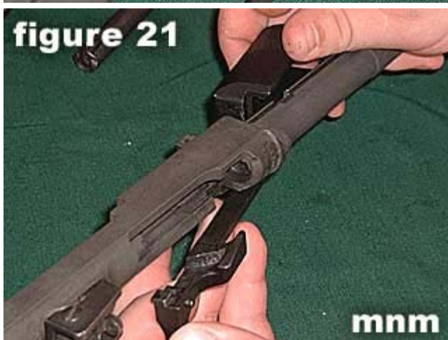
21) Figure 21 shows the correct way of removing the operating slide from the receiver.
