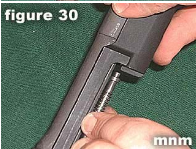
30) Place end of recoil spring guide into the guide hole as shown in figure 30.
