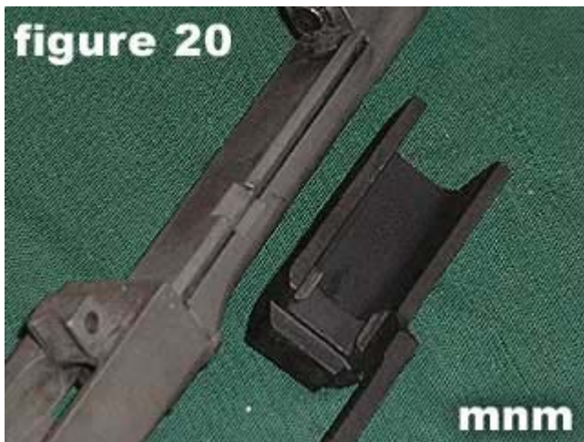
20) Figure 20 shows that the operating slide and how it aligns with the receiver. Note the notch in the receiver where you can slide the operating slide from the guide rails.
