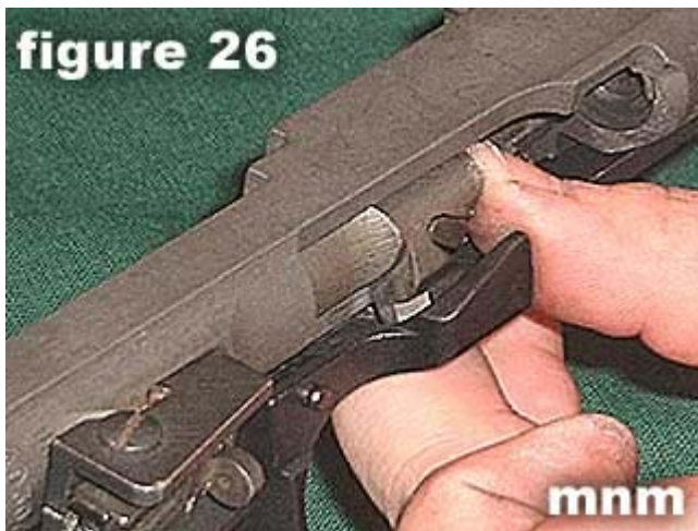
26) Connect operating slide to bolt as shown in figure 26.
