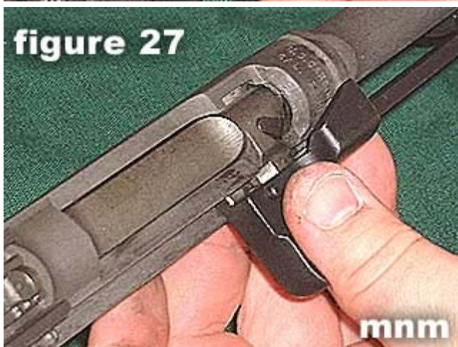
27) Carefully cycle operating slide and bolt to ensure no binding.
