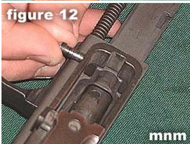
12) Remove the trigger guard pin and set it aside.
