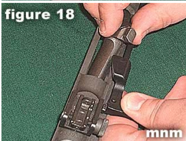
18) Pivot the bolt and remove as shown in figure 18.
