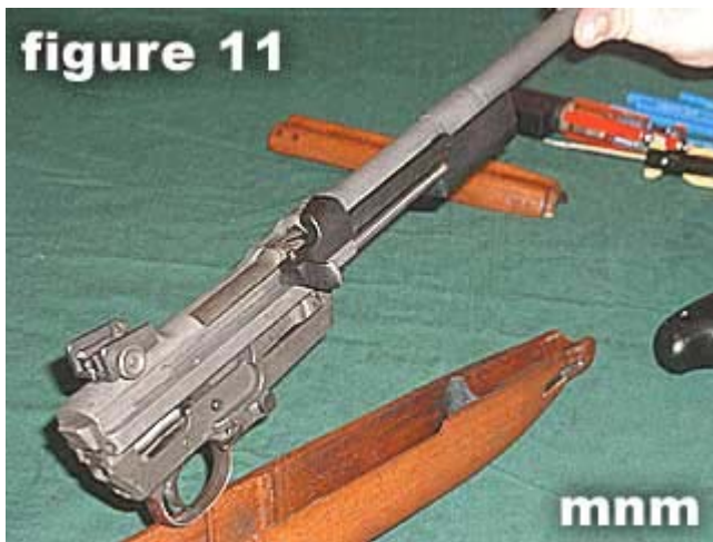
11) Remove the barrel and receiver from stock.
