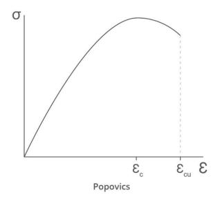
These have been adjusted and are based on the Thorenfeldt base curve. In the Canadian offshore code (CAN/CSA S474-04) this is characterised by
