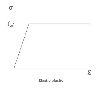
For some codes (CAN/CSA) the initial slope is reduced to  $\phi E$  .
