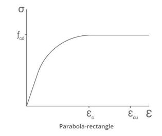
Parabola-rectangles are commonly uses for concrete stress-strain curves.
