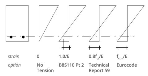
Integrating the stresses from this strain plane over the section will give an axial force equal to the applied force, and a moment which is parallel to the applied moment. The value of this moment is the cracking moment. Short-term material properties are always used for the cracking moment calculation.
