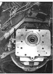
After the Torque Splitter was secured to a transmission jack, it was bolted into place on the bellhousing.
