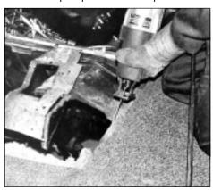
A hole was cut in the floorboard to make room for the overdrive shift lever and allow for the rearward (7-1/2 inch) displacement of the transmission/transfer case assembly and its two shift levers.
