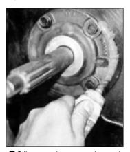
6 Silicone sealer was used around the edge of the retainer where it meets the transmission case so that oil would not pass between the transmission and the Torque Splitter.
