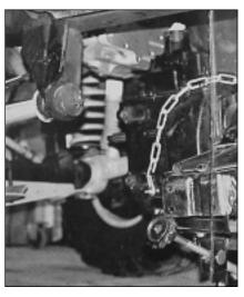
After fastening the transmission and transfer case to a transmission jack and securing the mass with a chain. The transmission is bolted to the Torque Spliter.
