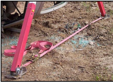
Attach strap from Baseplate to Baseplate or directly to the vehicle
