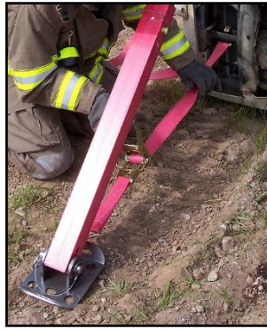
Attach strap from Baseplate to Baseplate or directly to the vehicle
