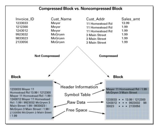
Figure 1: Compressed Block vs. Non-compressed Block
