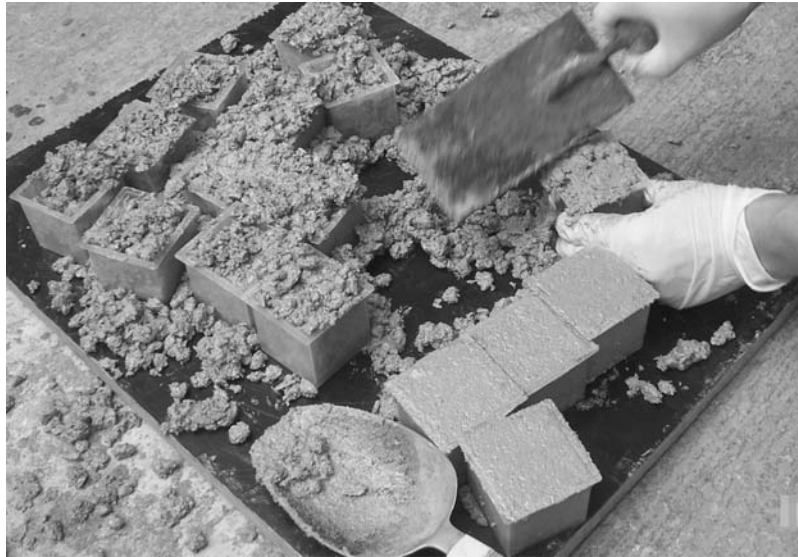
Figure 6-39 Casting of cubic specimens for determination of compressive strength
