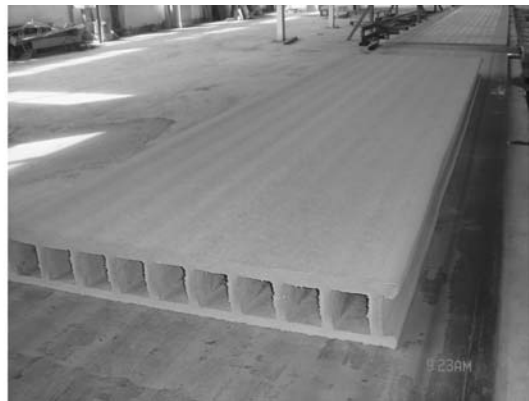
Figure 6-21 Extrusion process in a plant
