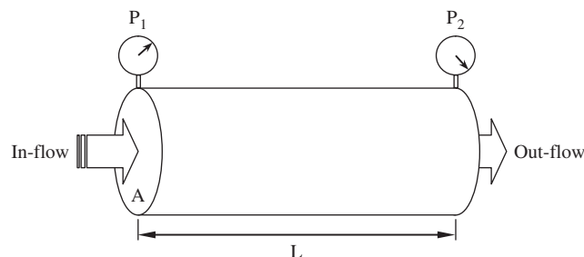
Figure 5-65 Steady-flow permeability test
