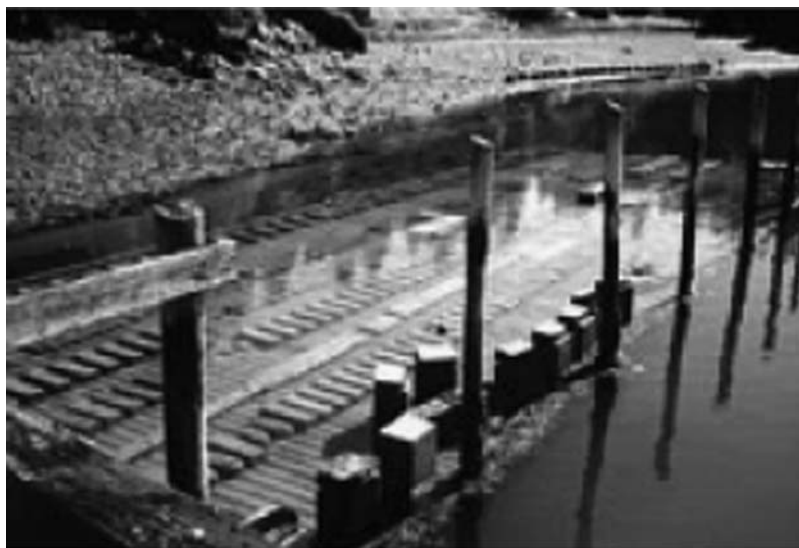
Figure 5-75 Storage pond for sulfate attack test
