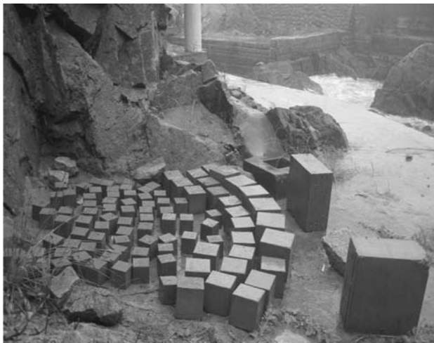
Figure 5-78 The marine exposure test site in Qingdao, China
