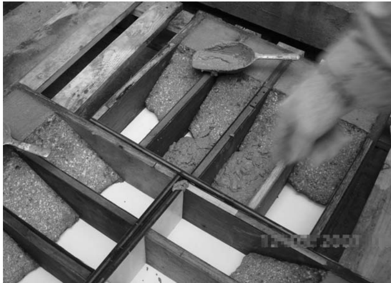
Figure 6-38 Casting of prisms for slant shear measurement
