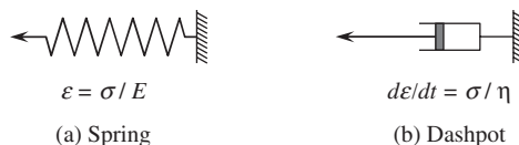
Figure 5-52 Spring and dashpot for modeling viscoelastic behavior
