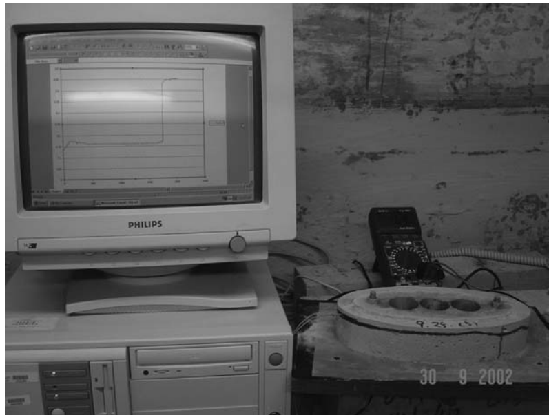
Figure 5-47 Elliptical ring test for constrained shrinkage
