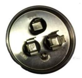
Notice that on the capacitors there are previsions for multiple connections. These connections are organized into groups of one to four connections. The "S" wire followed at the end of the previous step should connect to the HERM terminal on the three-terminal capacitor and one of the two terminals on the two-terminal capacitor. This terminal group on two terminal capacitors can be considered the HERM terminal group. The Orange wire from EasyStart must connect to HERM terminal group.
