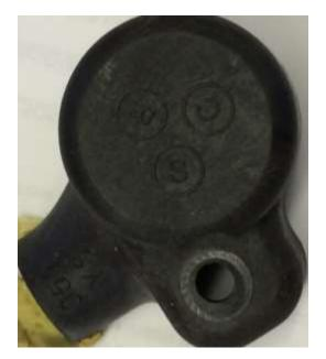
Some caps have the windings marked on the top as shown while others have markings inside the cap. Some compressors also stamp a letter on the compressor housing to indicate the connections.
