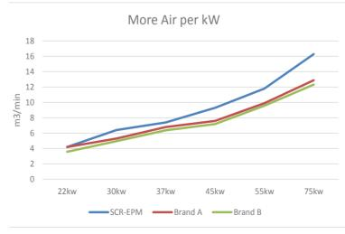
SCR have added a new high efficiency compression airend to the EPM series which delivers 10-15% more air. The size of the airend has also been increased and reaches optimum flow at significantly lower revolutions.
