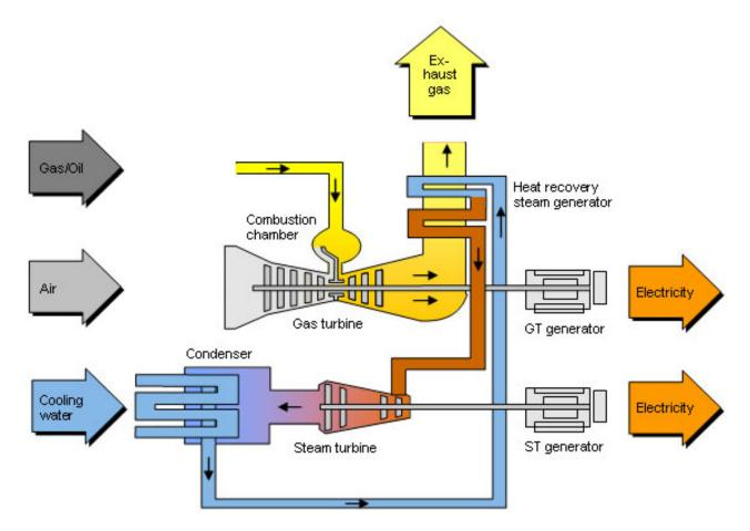
Schematic of large scale Combined Cycle Gas Turbine power plant from Siemens. Large scale plants of this type can be upwards of 300 MWe. Modern gas turbines are highly efficient with thermal efficiencies between 30 and 45%.
