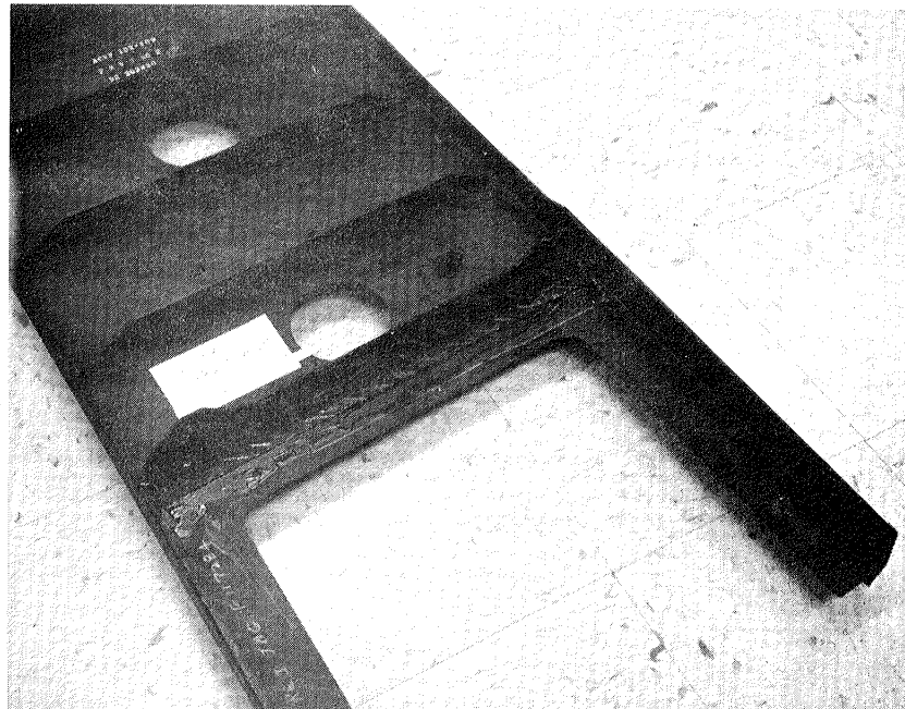
Figure 3-16. PRVT Spar Specimen No. 2, Ultrasonic Inspection Results - Crosshatched Areas Indicate Delamination
