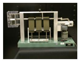
The B&R/TMI Testoflexer is an instrument for testing the flex life of shoe upper leather, coated textiles, and similar materials. It determines the number of flexing cycles that a material can withstand before it cracks in the creases, powders, or peels off in the folds.
