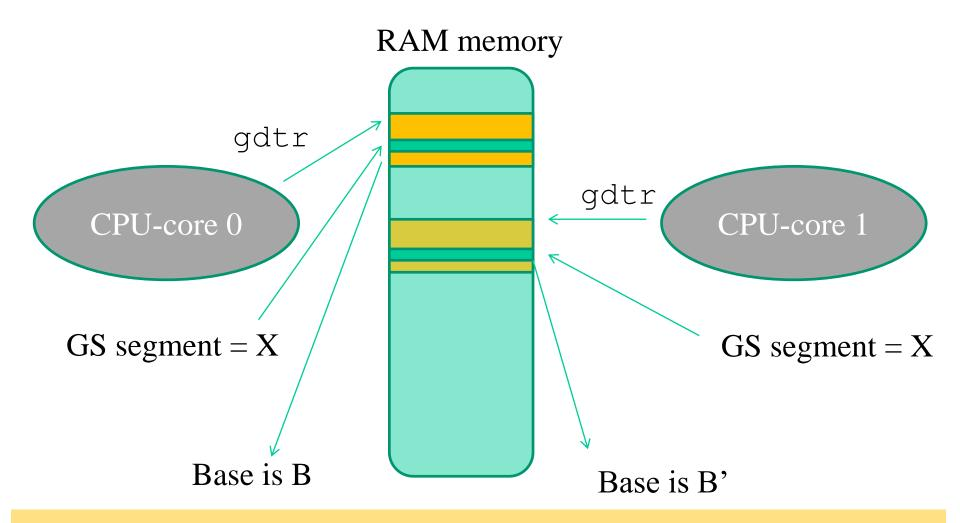
Same displacement within segment X seamlessly leads the two CPUcores to access different linear addresses
