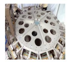
Qualitest spout sealing machine is automatic PLC controlled machine specially designed for mass production of packages with spouts and heat sealed packages.
