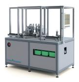
The revolutionary HDA consists of a hardness tester and a density measuring system which allows tests to be carried out automatically. This is an automatic system specialized for high capacity test.
