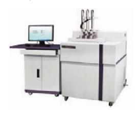
ASTM-D648, ASTM-D1525, ISO-75, ISO-306, DIN 53461, DIN 53460
