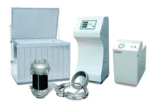
Conforming to ISO 1167 and ASTM D 1598 & 1599, the Hydrostatic Pressure testing system is mainly used to determine the resistance of thermoplastics pipes to constant internal water pressure at constant temperature.
