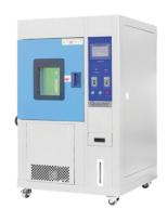
Ozone test chamber is a major factor in rubber cracking although it is rare in the atmosphere, ozone aging tank simulates and enhance the condition of ozone in the atmosphere to study the effects of ozone on rubber, and then identify and evaluate the method to resist ozone and aging for rubber, adopt effective anti-aging measures to enhance the life of rubber products.
