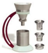
The Apparent Density Tester - Bulk Density Tester series testers are used to measure apparent density, bulk factor, and where applicable, the pourability of plastic materials such as molding powders. There are three methods according to ASTM D 1895 that are applicable to various forms of these materials that are commonly encountered - from powders and granules to large flakes and cut fibers. The apparatus consists of a measuring cup which is polished inside and a funnel.
