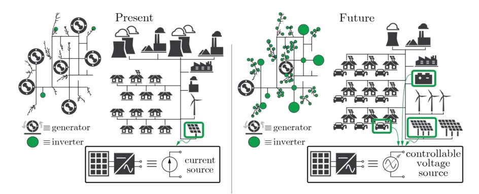
Synchronous generator based power system with inverters using gridfollowing controls To inverter dominated power system using next-generation grid-forming controls
