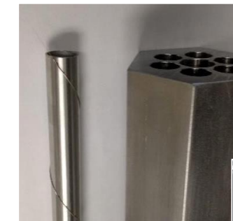
Distributed Fiber Optic Temperature Sensor on Heat Pipe
