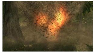
Particles drawn as hard billboards Soft particles Figure 4. Billboard and soft particle rendering comparison
