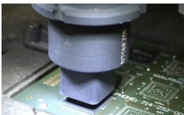
Figure 12. Standard Nozzle (Removes 1 Package at a time)
