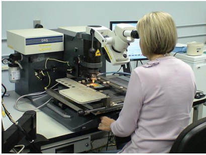
Figure 7. “Man”/Machine 01005 Rework Interface (MMRI)
