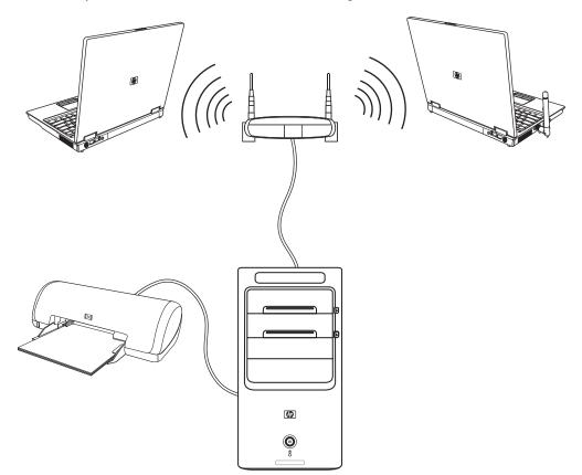
The preceding illustration shows a home LAN. The desktop computer has a wired connection to a wireless router. The desktop computer also has a printer that it shares with the other computers on the network. Each notebook computer has a wireless connection to the network router.
