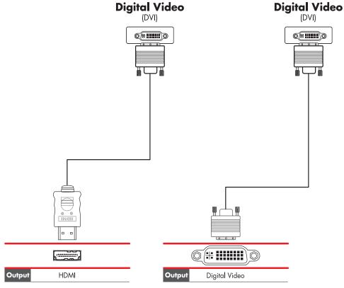
Connector on the Computer Connector on the Computer
