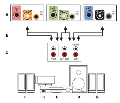
Computer to 5.1 multichannel audio system connection
