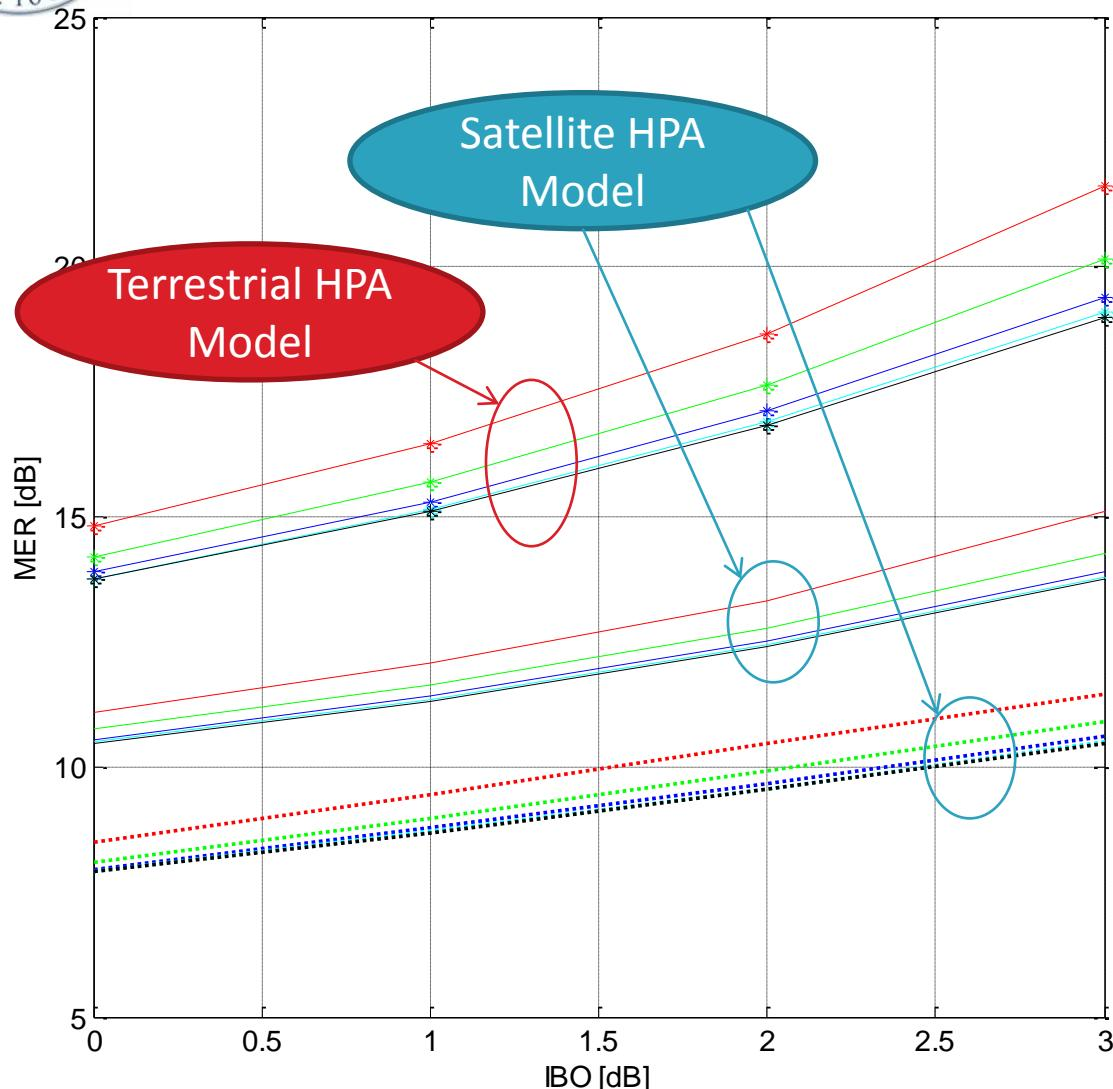
TWTA Model used in the DVB-SH standardization process Courtesy by ESA
