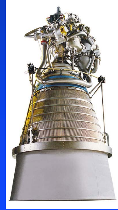
RL10 (Upper Stages) LH 2 /LOX Expander Vac I sp = 444 s Max. F vac = 23,500 lbf
