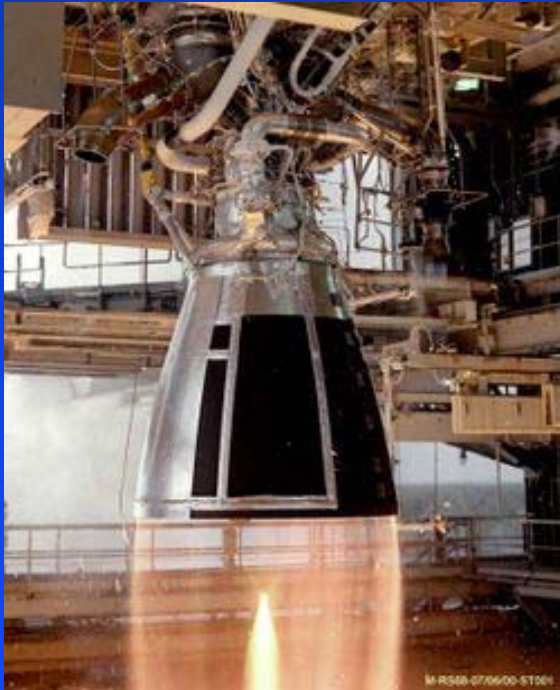
RS-68 (Delta IV) LH 2 /LOX Gas Generator Vac I sp = 410 s Max. F vac = 751,000 lbf
