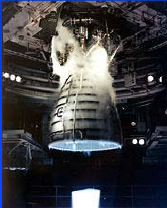
SSME (Space Shuttle) LH 2 /LOX Fuel-Rich Staged Comb. Vac I sp = 453 s Max. F vac = 513,000 lbf
