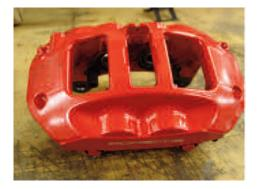
• Remove dust seals from the caliper pistons
