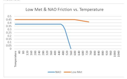
Low met performance characteristics are necessary to maintain the balance of performance in the Porsche vehicle as a whole.
