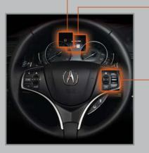
Roll the selector wheel to the tire pressure monitor to see which tires have low pressure.
