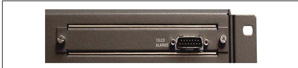
Figure 20: Shelf Alarm Panel (SAP)
