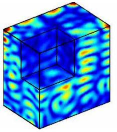
Instantaneous signal level will differ over time and with position in the chamber (Rayleigh faded signal) but the average over time is the same regardless of position in the chamber (within certain limits)
