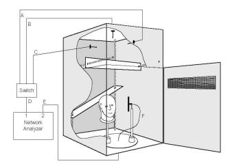
Isotropic field environment when averaged over large number of independent field samples
