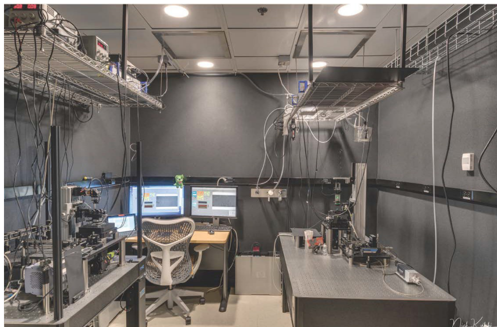
A pre-pandemic view of Neuman's custom-designed lab, specially calibrated for light, sound and motion: The room has two magnetic tweezers. At left, the instrumentation on the table is a magnetic tweezers that also incorporates fluorescence. The full instrument includes the electronics above the table on the rack and one of the computer monitors. The table on the right has a second magnetic tweezers on it. This one is a little more simple but all of the electronics on the right side of the room are part of the instrument, which is controlled by the second monitor on the table. This was all built by hand by the lab's staff scientist, Dr. Yeonee Seol, who often runs both instruments simultaneously from the dual monitor command center in the middle.
