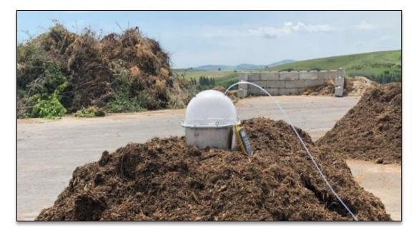
Figure 8: Photograph of flux isolation chamber at top of a 5% biochar pile.
