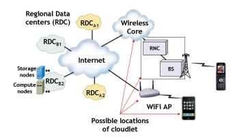
Figure 1: Components of mobile cloud architecture
