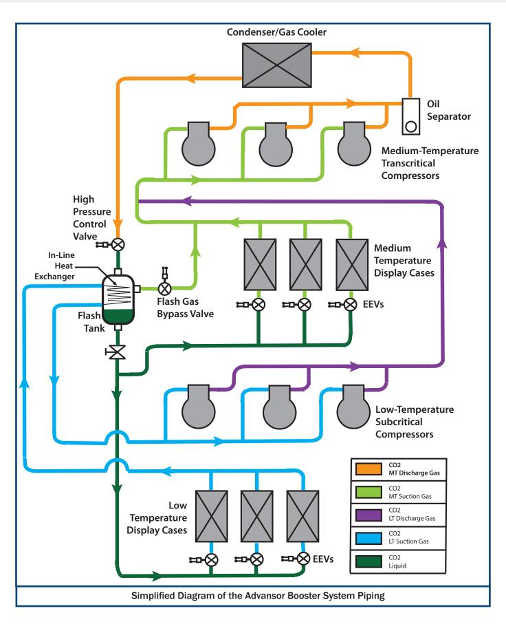
The sizing of the compressors on the low-temperature and medium-temperature stages of the system is carefully determined to provide optimal capacity control during partial load operation.
