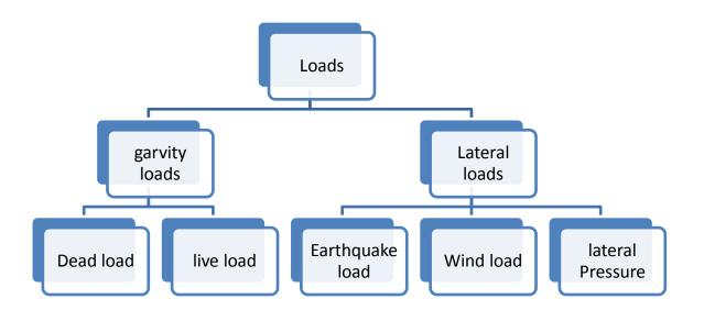
Gravity loads: Loads which acts in the direction of gravity i.e. towards the centre of earth.
