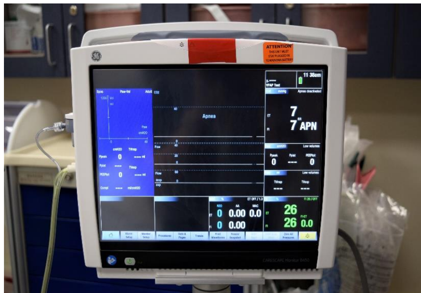
Figure 1. GE CARESCAPE™ B450 monitor. It can be mounted on a rollaway stand or placed on a sturdy surface (e.g. Mayo stand).
