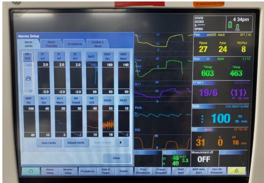
Figure 8. Alarms Setup. Note that the interface is slightly adjusted to view invasive airway pressures (See Section 4 – Additional surrogate monitoring).
