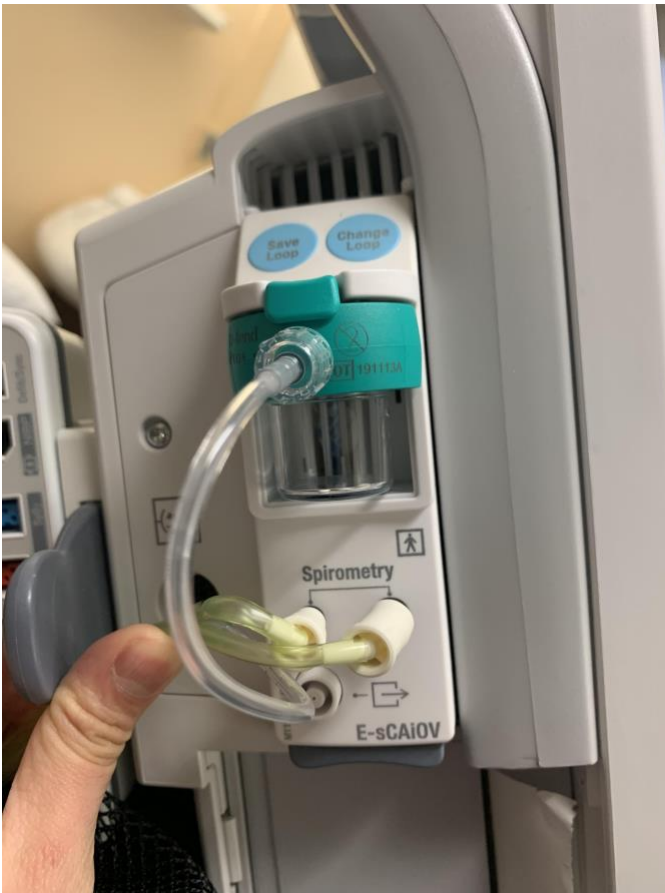
Figure 2: GE E-SCAIoV respiratory module with a D-Fend Pro+ side-stream gas sampling and spirometry
