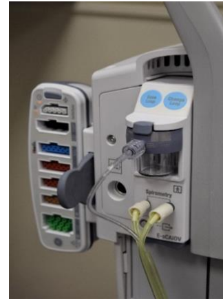
Figure 3. The back of the GE CARESCAPE™ B450 with the CARESCAPE PDM for vital signs, including invasive pressures. The E-sCAiOV module is also attached.
