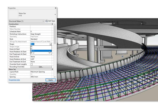
Improved rebar bending schedules for fabrication
