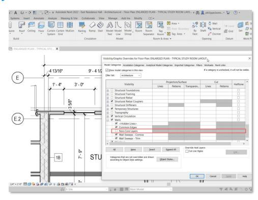
Quickly refine plan views to display wall core layers only
