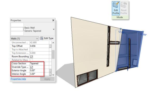
Improved wall modeling with tapered and slanted wall enhancements
