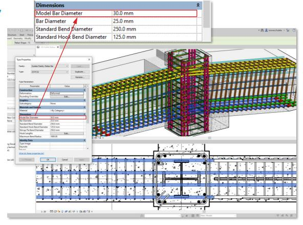
Improved user efficiency in modeling accurate concrete reinforcement
