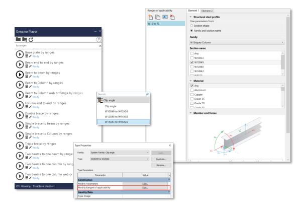
Place steel connections using predefined ranges of applicability
