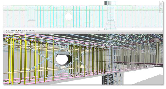
Improved user efficiency in modeling accurate concrete reinforcement
