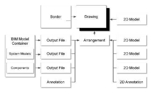
In the diagram above, the Output files are created from the BIM model to allow integration with the 2D CAD system. The drawing is then compiled in the 2D CAD system so that all designers have access to view and print the drawings, even if they do not have the BIM software installed.
