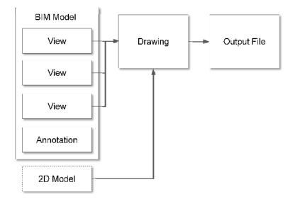
In the 100% BIM Workflow diagram, all views and annotation are created from within the BIM system. Additional 2D references may be attached as required. Output files are then exported from the drawing sheet for integration with 2D CAD systems or issue to external parties.
